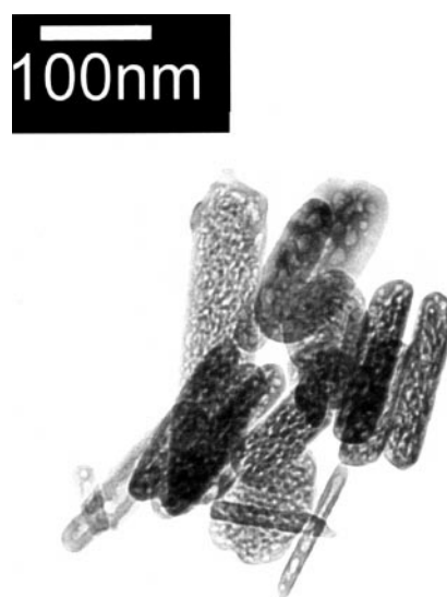
Fig. 11 Acicular crystals of tin-doped \alpha\text{-Fe}_2\text{O}_3 formed by heating tin-doped goethite at 370 °C (12 h).
